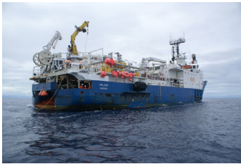
Combined source/cable/buoy handling vessel.
