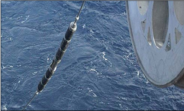
Figure 3 Cable for the OBC system being deployed.
